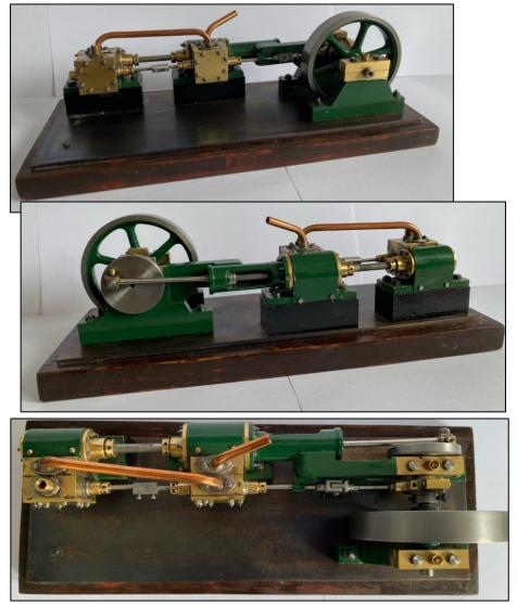
It goes without saying it runs perfectly once the engine has completed the first cycle and steam or compressed air has passed through the high-pressure cylinder and reached the larger low-pressure cylinder.
